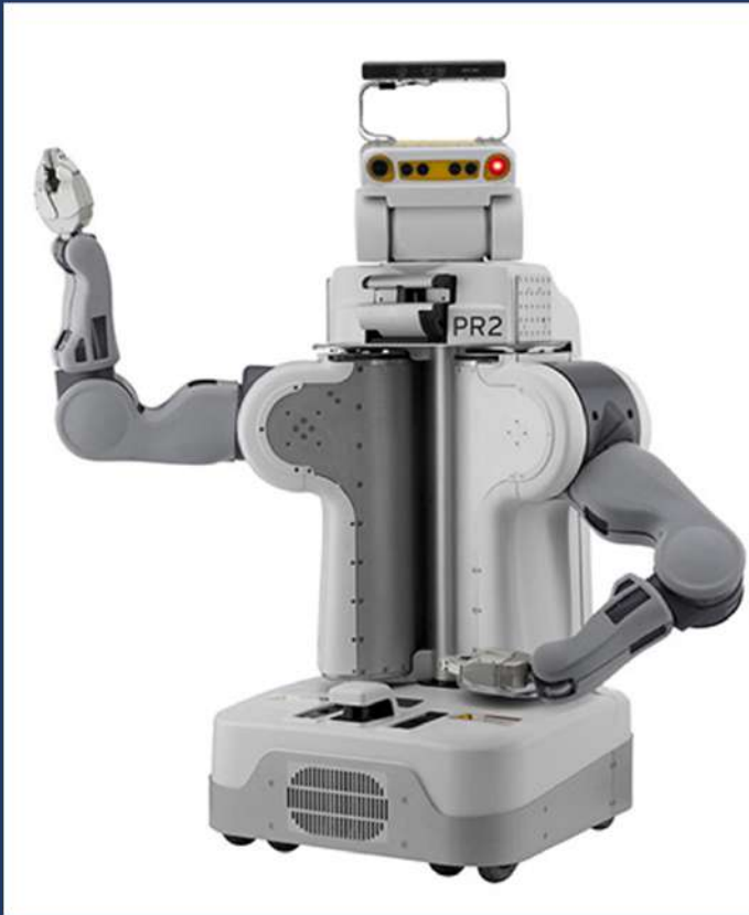
PR2: Built in 2010, weighs 500 lbs, cost $400,000
